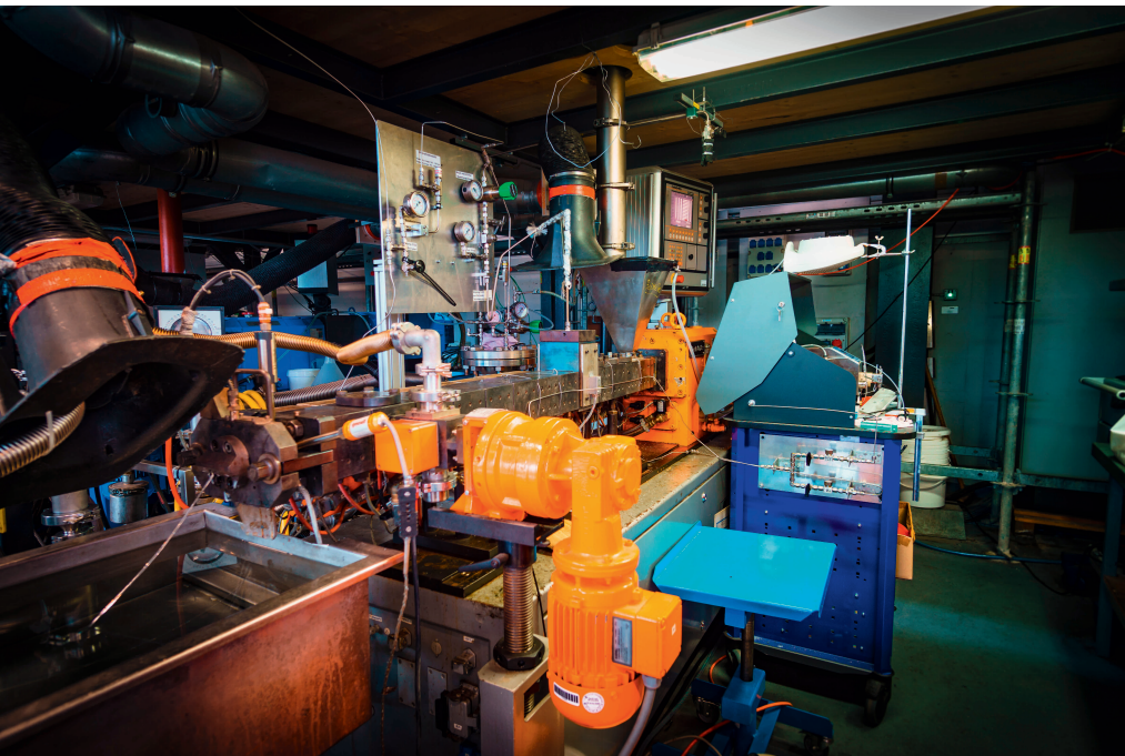
Pilotanlage zur extraktiven Extrusion am Fraunhofer ICT in Pfinztal. © Fraunhofer ICT
