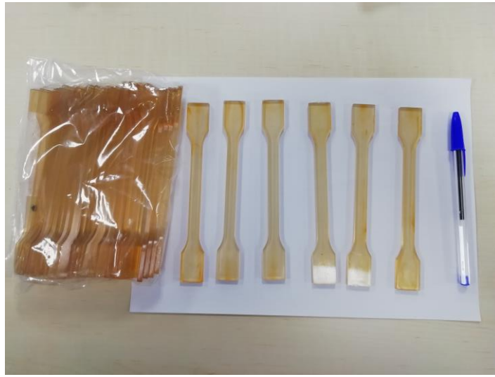
Figure 2. PS “dog bone” specimens
