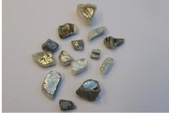
Figure 3: Metal-containing parts removed from ABS recycle.
