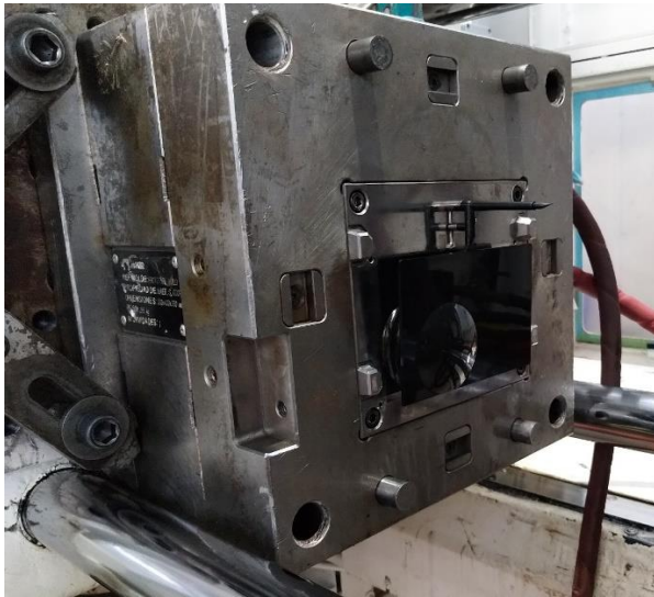
Figure 2: 2D injected demonstrator part on the mould
