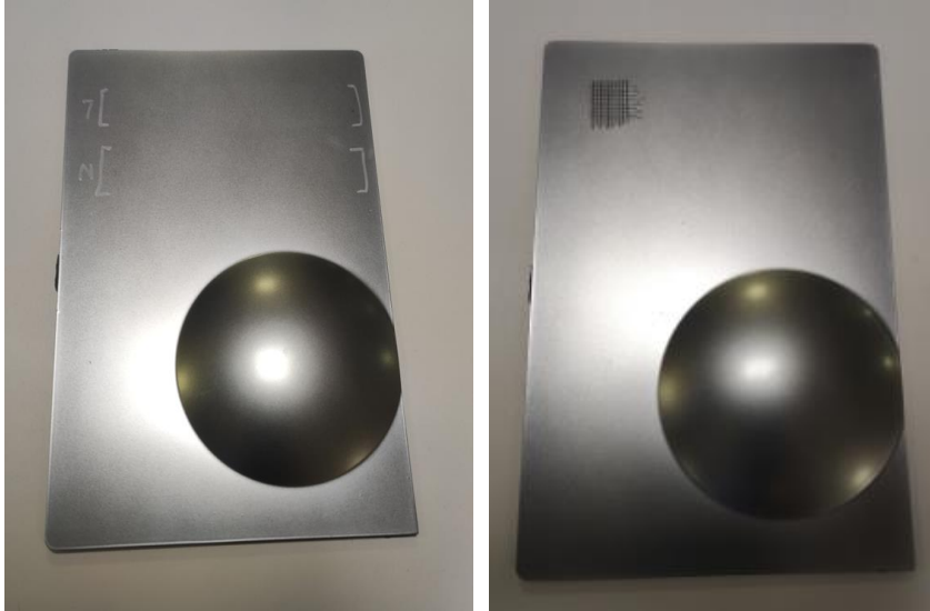
Figure 10: Left: Handcream and suncream tested demonstrator; right initial adherence tested demonstrator.
