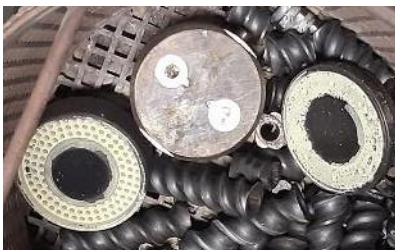
Figure 12: Contamination of spinning plate: cause of variations in extruder pressure
