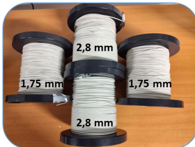
Figure 17: TGA White rABS filaments, additivated with 5 and 15% MAH.
