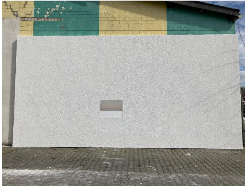
Figure 28: Completed test façade with a window for the CREAToR EPS in the middle.
