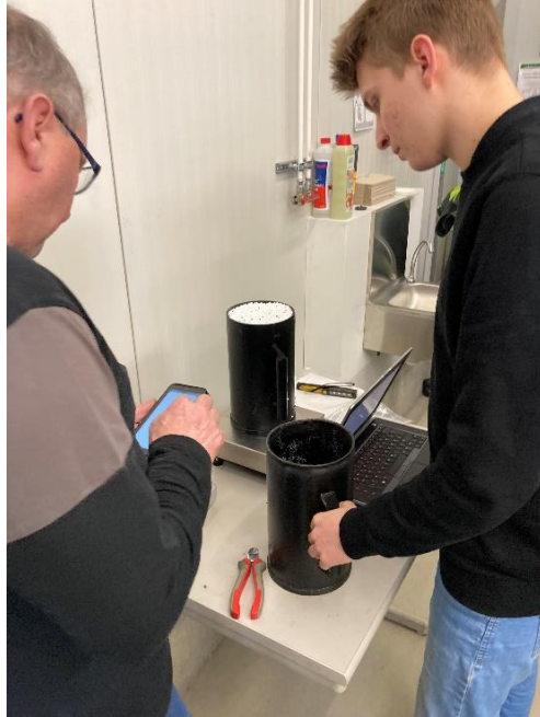
Figure 2: Measurement of the EPS density after pre-foaming for the purpose of optimising the process parameters
