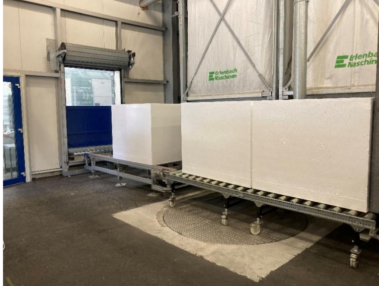
Figure 8: Three CREAToR EPS blocks produced during the trials
