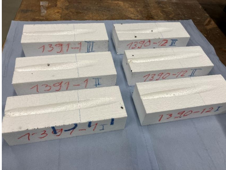
Figure 16: Every specimen passed the test for class E (DIN EN 13501-1)
