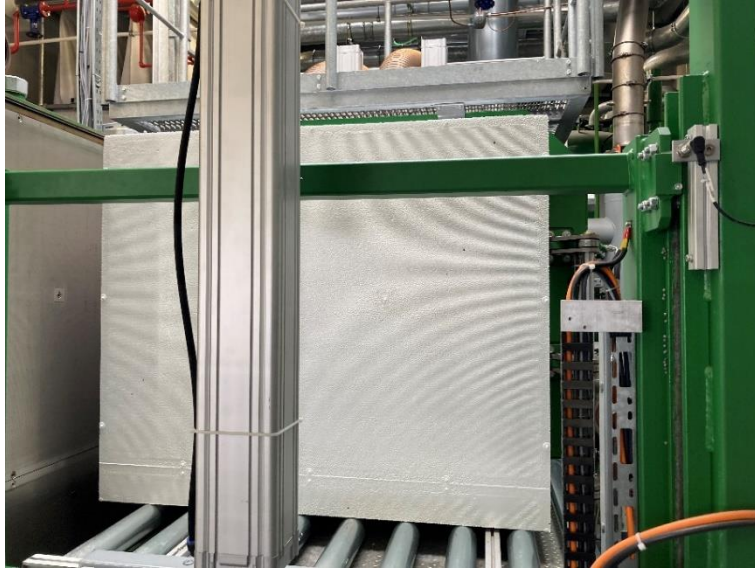
Figure 6: CREAToR EPS block ejected by the block molding machine
