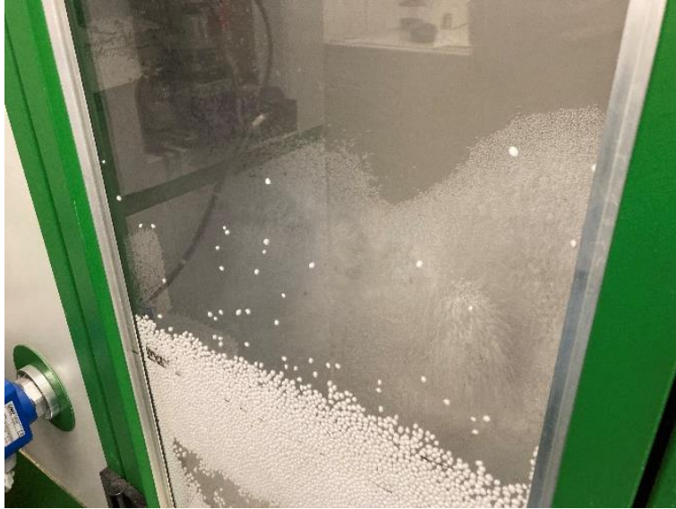
Figure 4: Collection container for the expanded PS beads (material is stirred up to prevent sticking)
