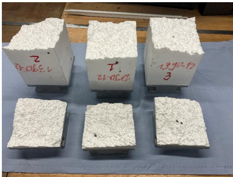
Figure 13: Fracture pattern of the test specimens
