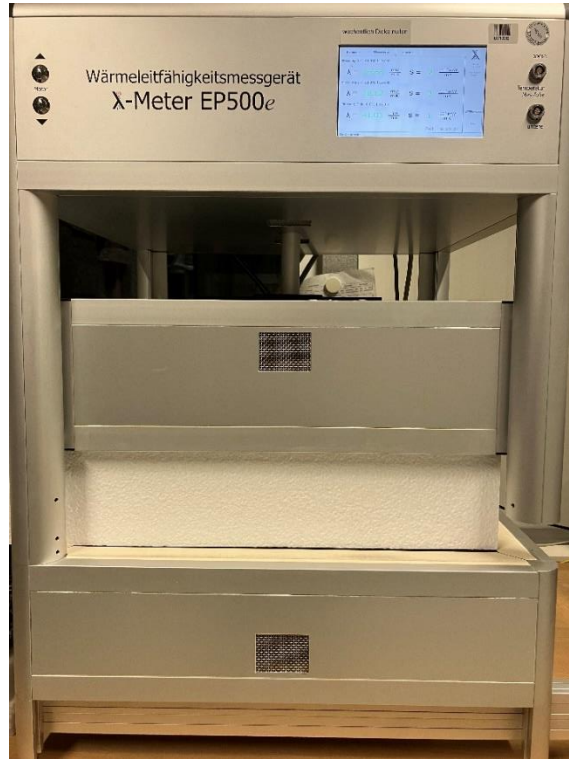
Figure 11: Measurement of the thermal insulation properties
