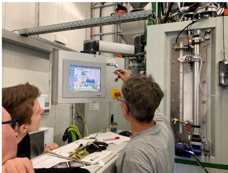
Figure 3: Setting of the parameters with running pre-foaming process (see right side)
