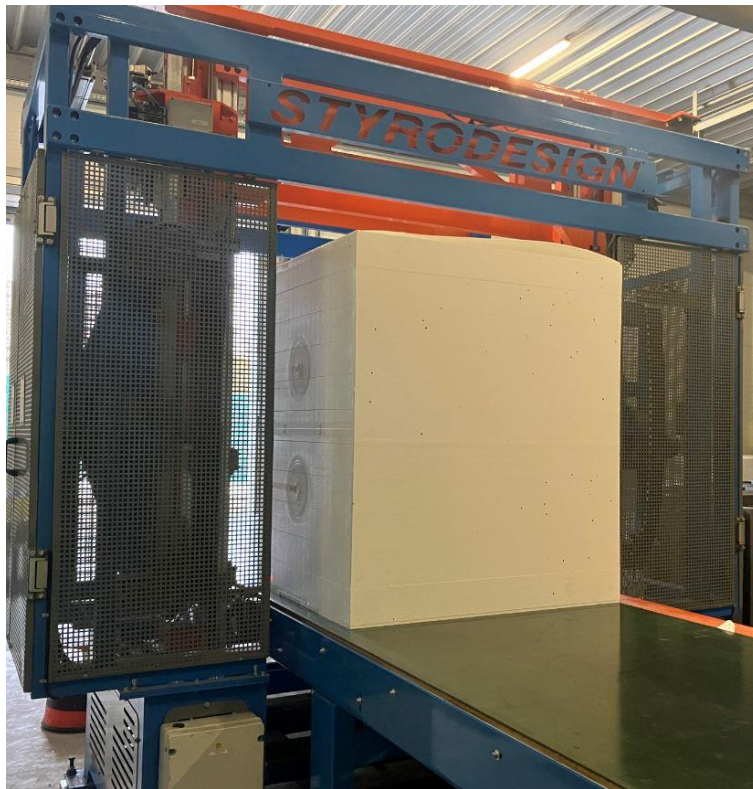
Figure 9: Cutting the EPS block into thermal insulation boards (500x1000x12 cm)
