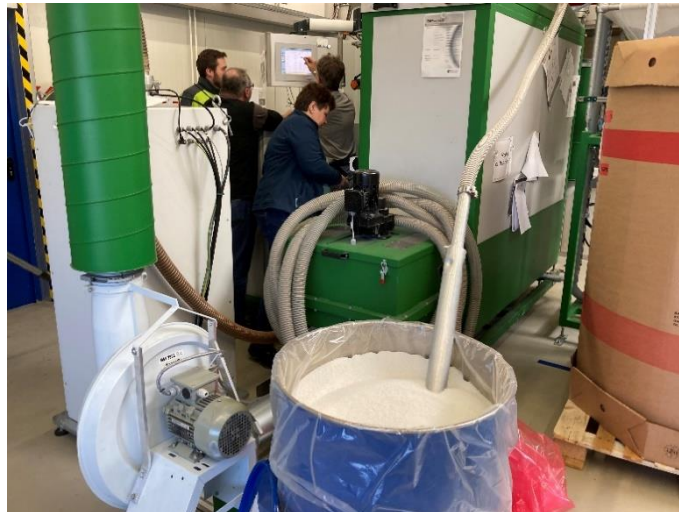
Figure 1: CREAToR polystyrene raw material (front) with nozzle intake for pre-foaming
