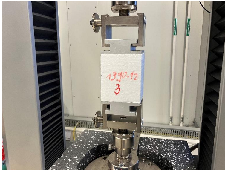
Figure 12: Measuring the tensile strength
