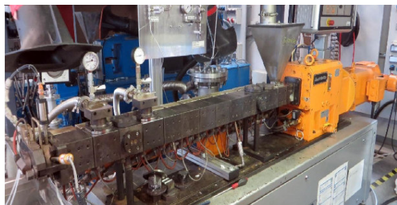
Figure 2 CREAToR extrusion process (real process on the left and schematic view on the right)
